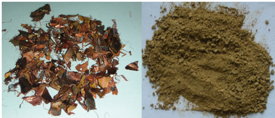
Fig. 3. Photographs of reaction products after lixiviation of the solidified salt, i.e., metallic fraction (left) and brown powder (right), respectively.
